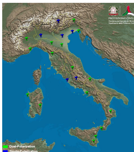
Figure 13: The radar network of the Department of Civil Protection. Green radars operate with dual-polarisation, blue radars have single polarisation.
