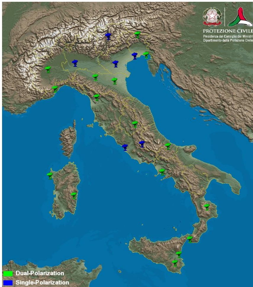
1200 Figure 13: The radar network of the Department of Civil Protection. Green radars operate with dual-polarisation, blue 1201 radars have single polarisation.
