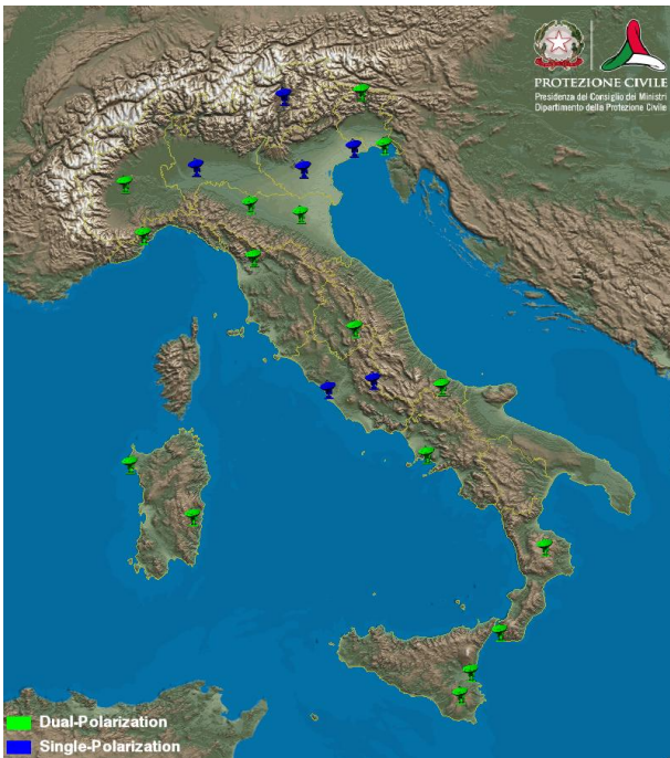
Figure 13: The radar network of the Department of Civil Protection. Green radars operate with dual-polarisation, blue radars have single polarisation.
