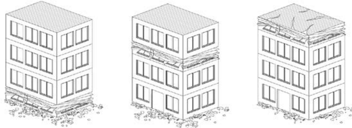
Fig. 1. Single-story collapse. Copied from So (2016).
