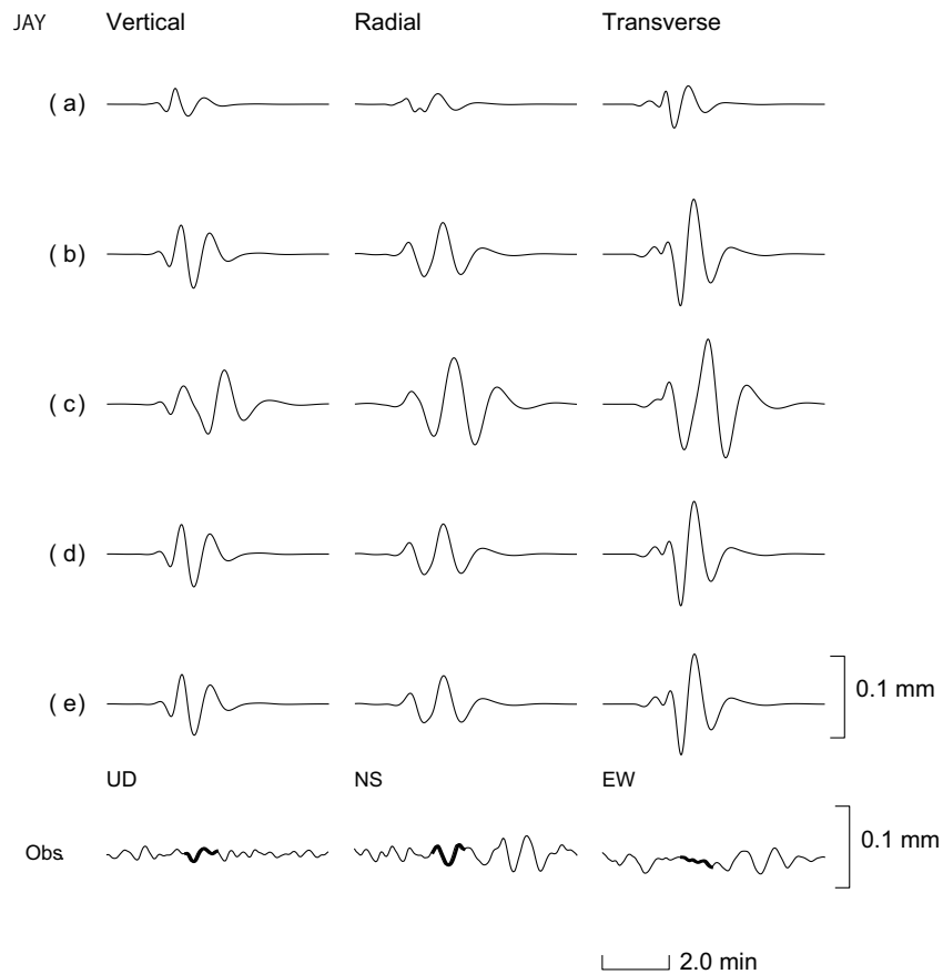
Figure 5. Synthetic seismic records constructed to represent the signature of the submarine landslide as it would have been recorded at station JAY, 176 km from the landslide source area (Fig. 1). The vertical and radial components are as viewed at an observation point along the assumed force direction. The transverse component is as viewed at an observation point on a line perpendicular to the direction of the source force. Different source-time functions were assumed for (a) to (e), as shown in Table 3. The seismic data recorded at station JAY 12.5 min after the mainshock are also shown (bottom panel). The bold parts of the observed records correspond to those in Figs. 3. A 50–100 s bandpass filter was applied to all records shown.
