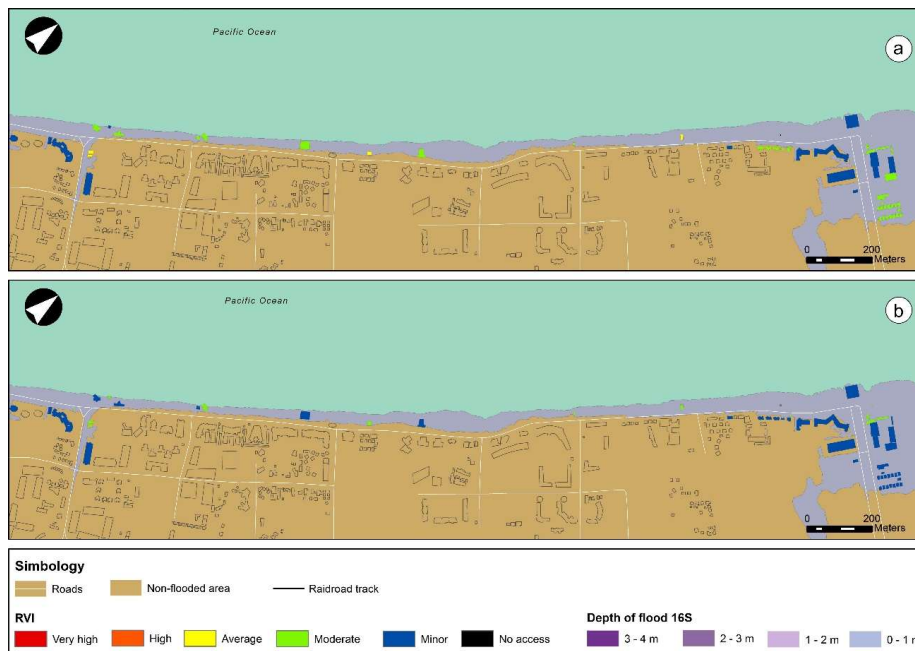
Figure 10: Relative Vulnerability Index for Sector 6 - La Serena: a) PTVA-3 model; and d) PTVA-4 model.
