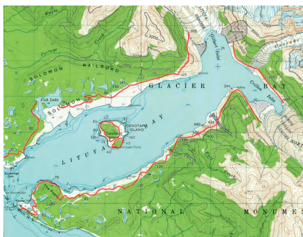
Figure 1. Topographic map of Lituya Bay (U.S. Geologic Survey, 1961) showing the settings and trimline of 1958 megatsunami (based on data from Miller (1960)). Units in feet. Key locations as Gilbert and Crillon Inlets, Centotaph Island, Fish Lake or The Paps are shown.
