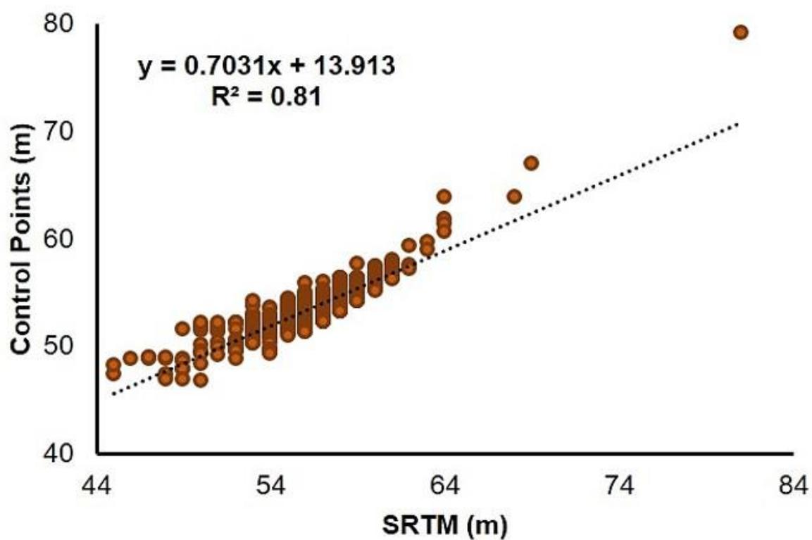
Figure 5: Linear regression analysis of SRTM image vs Ground Control Points (GCPs).
