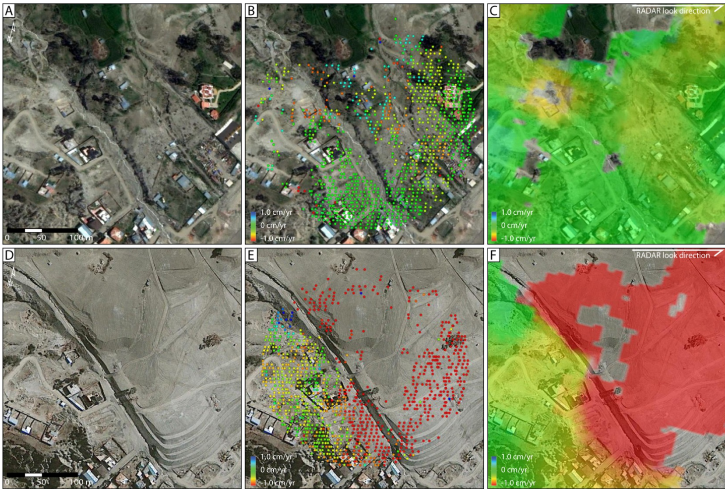
5 Figure 7. Typical density and spacing of HDS-InSAR results for an area of mixed suburban, agricultural, and commercial development. Both the pre-failure stack (A, B, C) and post-failure stack (D, E, F) are shown. Panels For each stack depict: satellite image showing land cover without InSAR data (A, D); point data representing HDS neighbourhoods (pixel neighbourhoods) (B, E), each recording a displacement time history; and linear displacement map interpolated from HDS points (C, F). Localized variability in HDS results is suppressed by linear deformation interpolation. Displacement rates are in the satellite line of sight. The deforming area is the southern boundary of the active part of the landslide toe (see Fig. 7 for location). Base image is a 4 January 2011 Quickbird image viewed in GoogleEarth™. Base images are from GoogleEarth ([A, B, C] 4 January 2011 and [D, E, F] 25 July 2011). See Fig. 8A, C for location.
