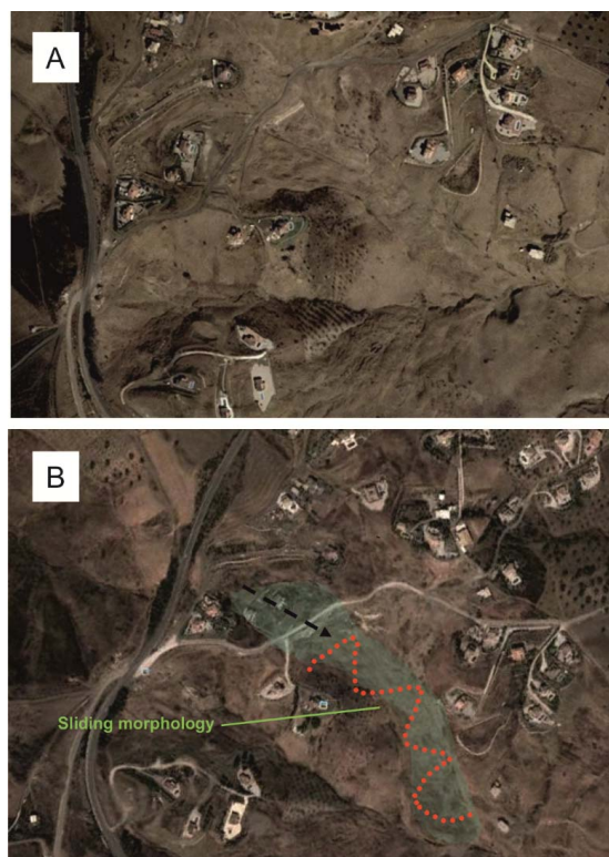
275 Figure 5. A) An aerial photograph from before the event (2006). B) An aerial photograph taken after the 276 landslide (2010).
