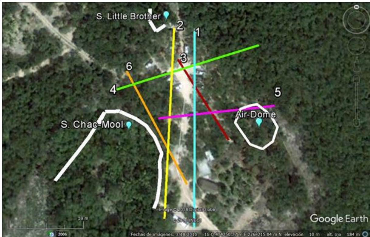
Figure 2. EM survey on the Chac-Mool sinkhole. Numbered profiles crossing the hidden rivers. With white wide line are the sinkholes exposed
