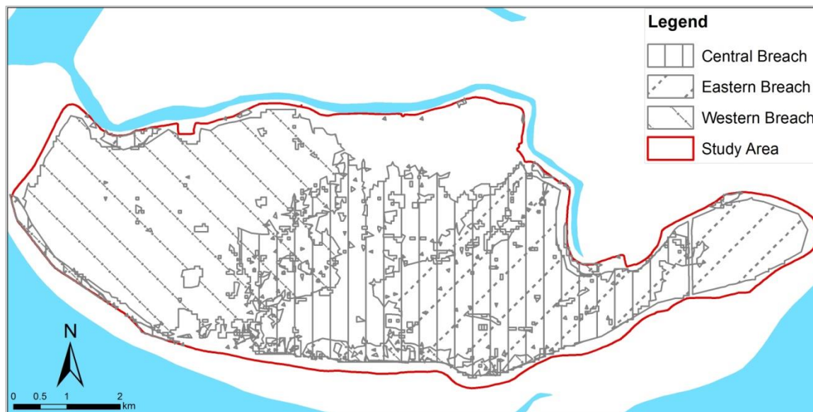
Figure 4: Flood extent corresponding to three worst case scenarios of dike breaching in the central, eastern and western section of the dike.
