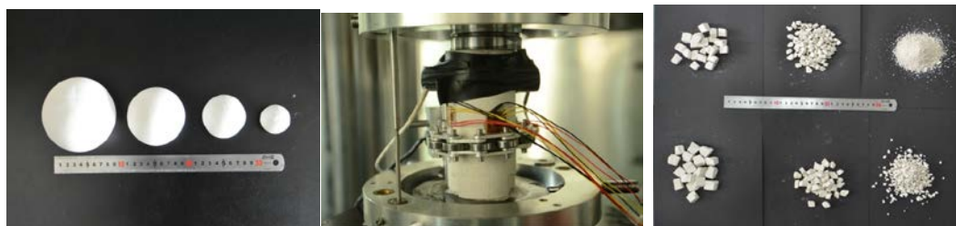
131 132 (a) Spherical gypsum samples of different sizes (b) Standard specimen under a uniaxial compression test (c) Sieved granules of different particle sizes 133
