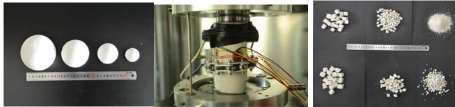
(a) Spherical gypsum samples of different sizes (b) Standard specimen under a uniaxial compression test (c) Sieved granules of different particle sizes
