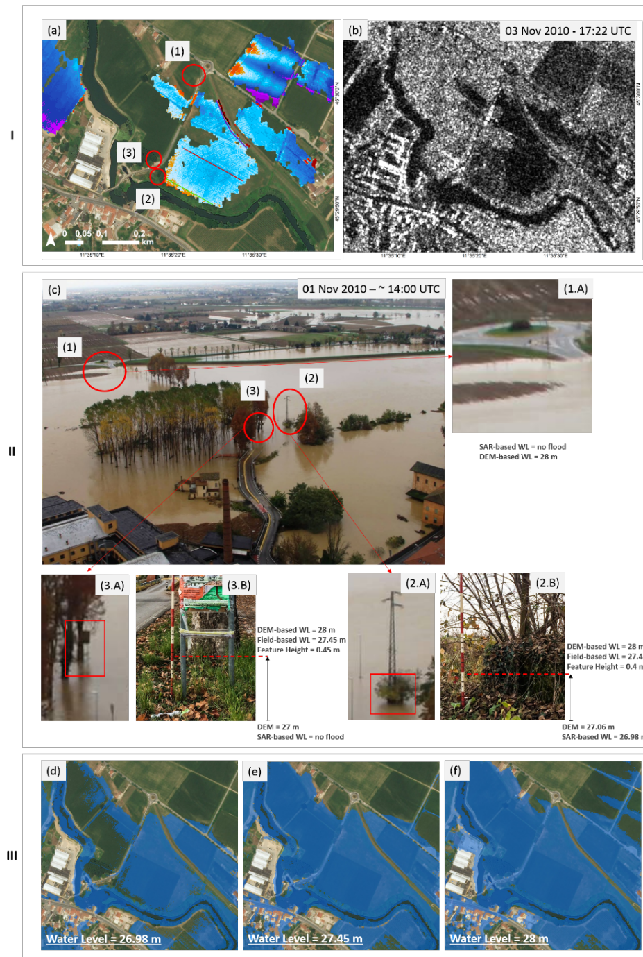
410 Figure 9 Flood depth on November 3 over Ponti di Debba in the Vicenza area of interest; panel I shows (a) flood depth on the area analysed; (b) CSK image acquired on November 3 at 17:22 UTC from where the flood map has been derived; panel II shows (c) aerial view of the event acquired on November 1 at about 14:00 UTC with zooms on three areas (1.A, 2.A, 3.A) with relative fieldwork images (2.B and 3.B); panel III shows the flood extent derived with the DEM-fill method for different water levels: (d) with water level equal 26.98 m corresponding to the level estimated by the proposed method; (e) with water level equal to 27.45 m, corresponding to the water level estimated by fieldwork data; (f) with water level equal to 28 m, corresponding to the level estimated by the DEM-fill method in order to obtain the same flood extent of the aerial photo.
