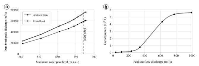
Figure 6: (a) Example of relation between the maximum water level attained in the reservoir and failure peak discharge, depending on the failure mode considered (abutment or central break). (b) Example of discharge-consequences curve.
