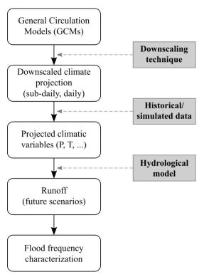
5 Figure 4: Synthesis of the methodology for the frequency analysis of floods under climate scenarios.
