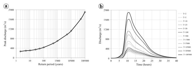
Figure 2: (a) Example of flood frequency characterization, used in the Flood node. (b) Resulting hydrographs, used for the flood routing computation.
