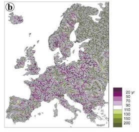
Figure 3: (a) Multi-model median return period (years) in the 2080s for the 20<sup>th</sup> century 100-year flood based on one hydrological model driven by 11 GCMs under RCP8.5 (from Hirabayashi et al. (2013)). (b) Change in recurrence of a 100-year flood in Europe in H12A2 scenario run using a Gumbel distribution (from Dankers and Feyen (2008)).
