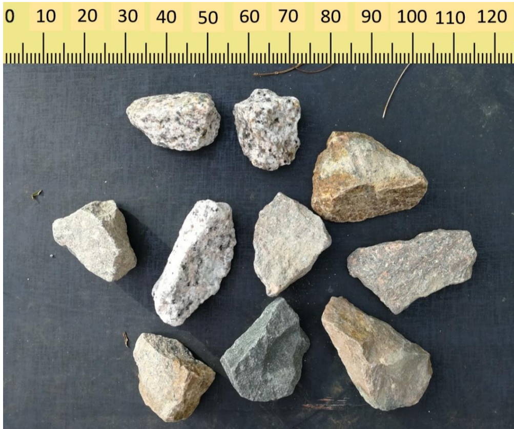
Figure 4. Aggregate samples in the granular flow impact tests (unit in mm)
