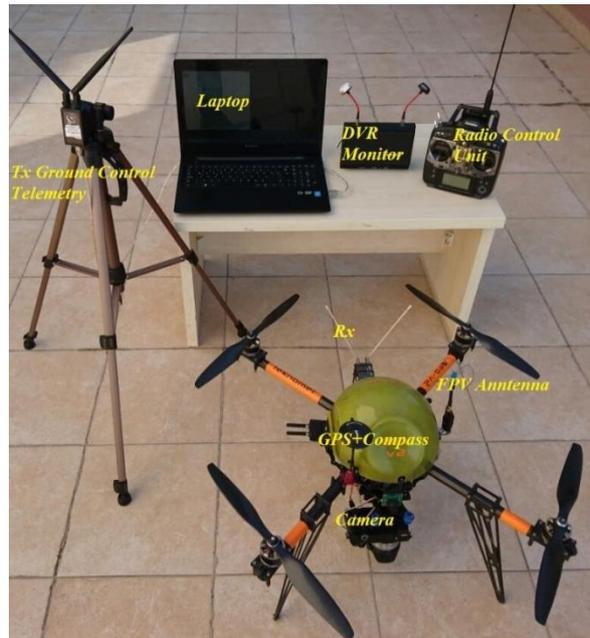
Figure 2. UAV environmental components
