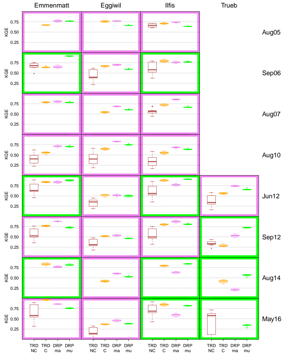
Figure 4. Re-analysis of eight large runoff events from 2005 to 2016 with CombiPrecip data in the four Emme catchments. The boxplots represent the simulation results of the different model configurations. TRD-NC stands for uncalibrated PREVAH, TRD-C for calibrated PREVAH, DRP-ma for RGM-PRO relying on Margreth map and DRP-mu for RGM-PRO based on Müller map. Border color reveals whether DRP-ma (pink) or DRP-mu (light green) performed better in terms of median KGE. Where no boxplot is visible, all KGE values were below zero. The spread in KGE of uncalibrated PREVAH results from ten random hydrological parameter sets out of 4'000 Monte Carlo simulations, whereas uncertainty from calibrated PREVAH originates from the ten parameter sets with highest KGE for the May16 event in Emmenmatt. Spread in RGM-PRO arises from simulations with ten hydrological parameter sets lying in narrow ranges determined by sprinkler experiments (Antonetti et al., 2017).
