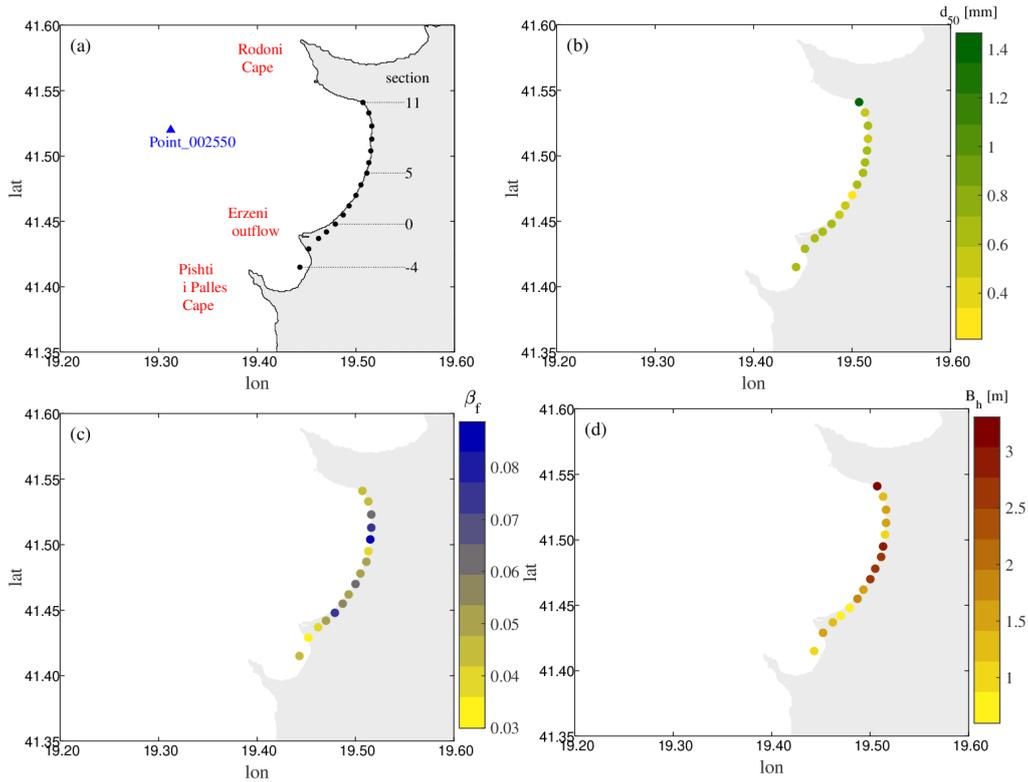
**Figure 3.** a) Sampling locations for beach sections (from -4 to 11, from south to north), Point\_002550 represents DICCA wave hindcast. Spatially distributed values of: b) Median grain size ( $d_{50}$ ); c) Cross-shore mean slope ( $\beta_f$ ); d) Berm height ( $B_h$ )
