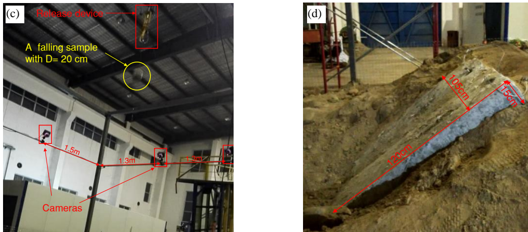
Figure 3. The testing apparatus in this study. (a) A general view of the apparatus. (b) A schematic representation of the specifically designed release device. (c) A falling sample after the wireless switch was turned on. (d) Slabs to be replaced for excessive damage.
