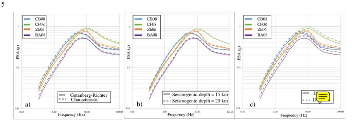
Figure 5 : Impact of the different uncertainties explored in the logic tree on the UHS at 10,000 years for the site of interest. From left to right: Shape of the MFD, Seismologic depth and Dip of the faults.
