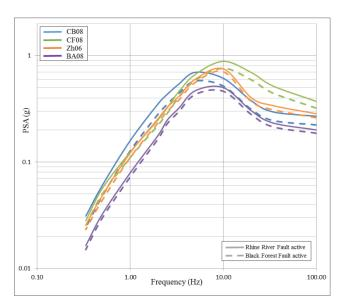
**Figure 6:** UHS at 10,000 years return period considering four GMPEs : CB08, CF08, ZH06 and BA08 (see Table 3 for references). Seismogenic depth of **15km**, the steepest dip of faults, the slowest slip rate, a Gutenberg-Richter frequency-magnitude distribution, the seismic moment method and  $\mu$ =3 10<sup>10</sup> N.m<sup>-2</sup>.
