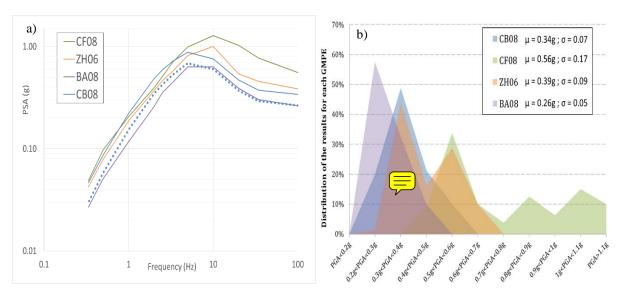
Figure 2 : Left: Uniform Hazard Spectra for a return period of 10,000 years. Mean UHS of the logic tree in black. Mean UHS for each GMPE in color. The dotted line is the branch used for the sensitivity analysis. Right: dispersion of PGA at 10,000 for each GMPE branch resulting from the exploration of epistemic uncertainties shown in Figure 1.
