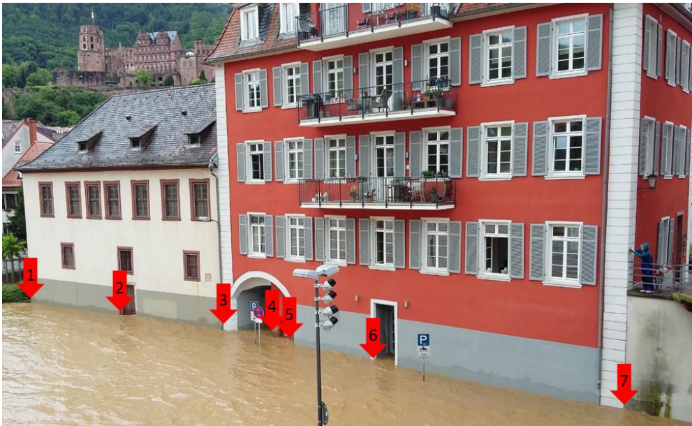
Figure 2: Example flood image with reference positions for manual in-field inundation depth measurements at the study site indicated with red arrows.
