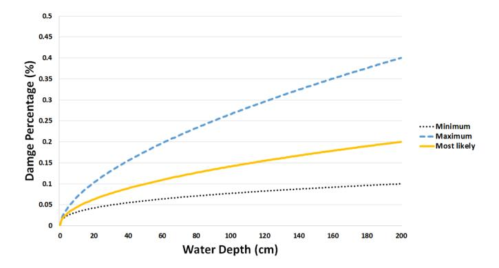
Figure 4. Visualisation of minimum, most likely and maximum damage functions, calculated by bootstrap and chi-square test of goodness of fit.
