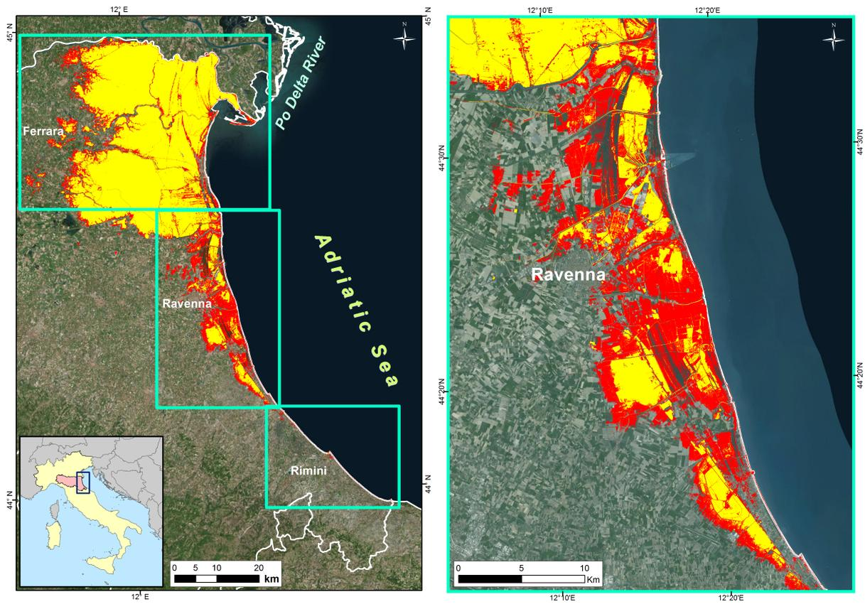
**Figure 5.** Results for the simulations in CS1, at the E-R coastal plain scale (left) and for the area of Ravenna (right). Lands that are currently located below sea level are evidenced in yellow. New areas predicted to be located below sea level at 2100 are marked in red.
