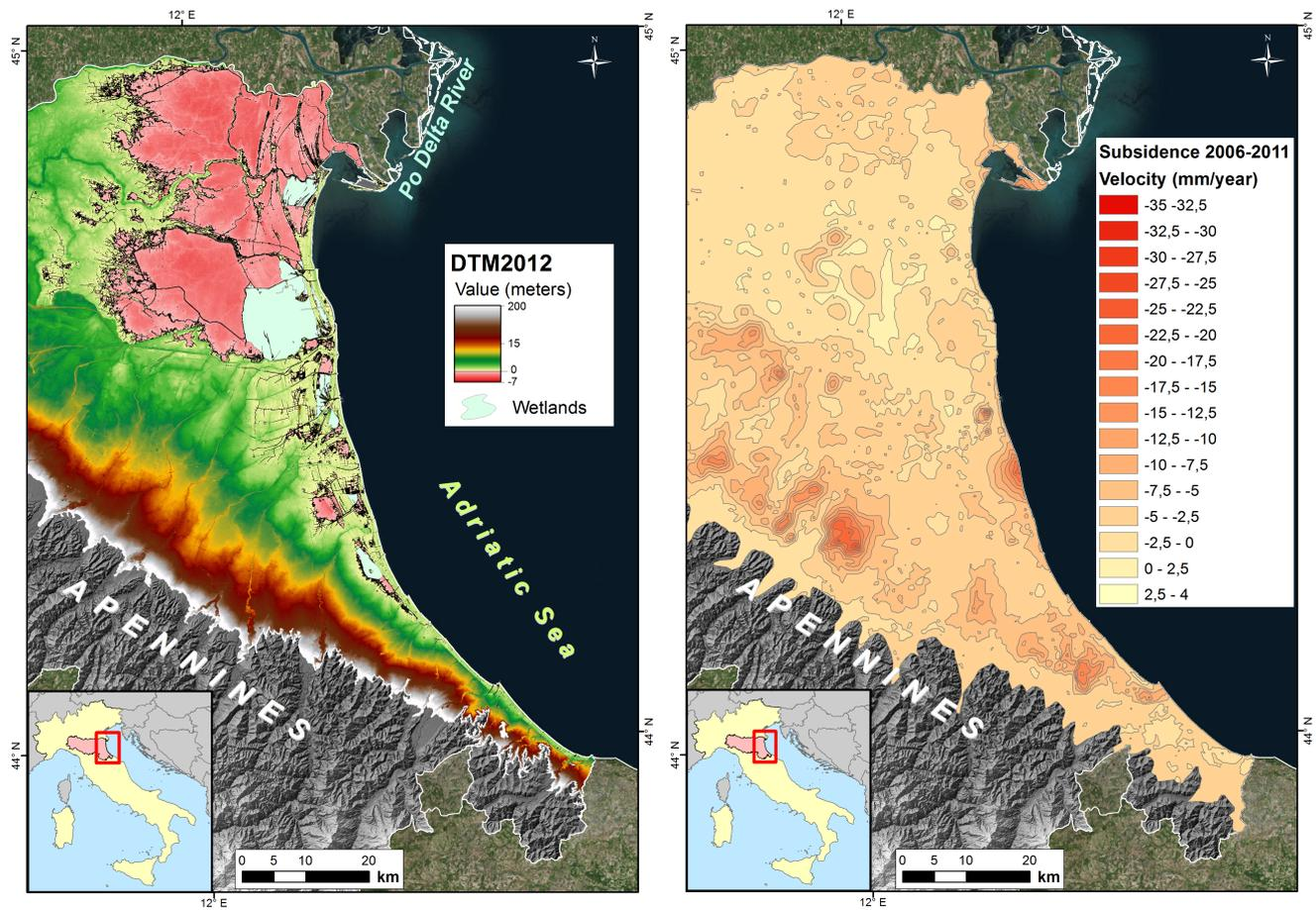
**Figure 2.** Left: the altimetry and morphology of the E-R coastal plain resulting from a high resolution Digital Terrain Model (DTM). The reference height in the map is the zero of the Italian geodetic network. The remarkable difference between the N and the S sectors in term of the extension of low lands is evident. Right: Subsidence rate map of the E-R coastal plain according to the InSAR monitoring for the time period 2006-2011 (Arpa-RER, 2012).
