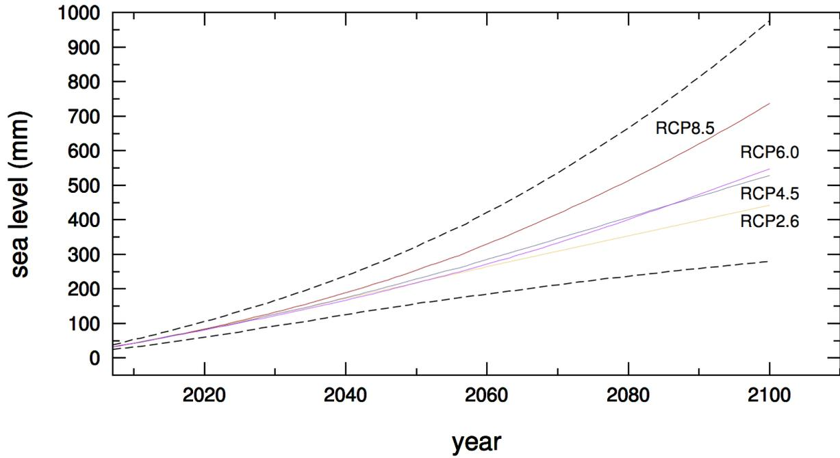
**Figure 3.** Sea-level pathways according to IPCC AR5. Dashed lines show the lower and the upper limits of the projections, corresponding to the upper limit of RCP 8.5 and to the lower limit of the RCP 2.6. Projections are referred to the average sea-level values in the period 1986-2005.
