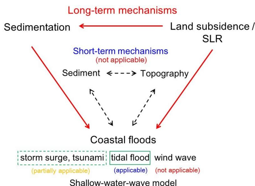
**New figure to be inserted in the revised manuscript:** Scope and the applicability of the proposed model. Long and short-term mechanisms could both cause morphology changes of a mangrove embankment. However, only the long-term mechanisms were taken into consideration in this study. The shallow-water wave model adopted here can reproduce the propagation of not only tides but also storm surges and tsunamis over the embankment. However, the latter mechanisms may not be always reproduced.
