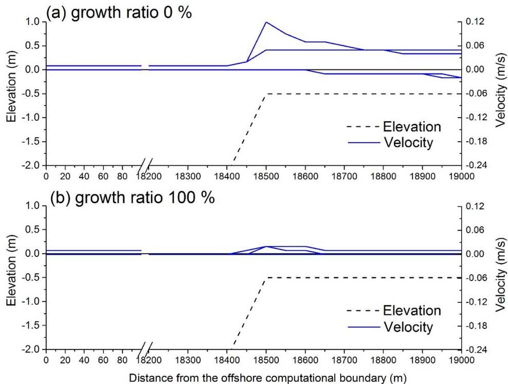
**New figure to be inserted in the revised manuscript:** Cross-sectional profiles of flow velocity during one tidal cycle (line was drawn every 6 hours). The water depth of the embankment was assumed 50 cm.
