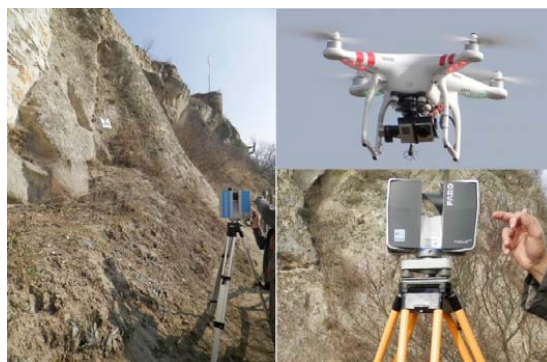
Figure 5. Applied remote sensing techniques (clockwise): Z+F Imager; 5010C DJI Phantom 2 with the GoPro Hero3+ action camera and Faro Focus S 120 3D
