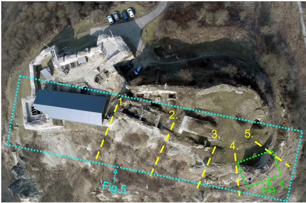
Fig.3. Location of the illustrations in the paper and the sections (1 to 5 marked by yellow dashed lines) where slope stability was calculated by using 2D FEM model (Fig.8). Dotted lines indicate the areas shown on Fig. 4 and Fig. 7.
