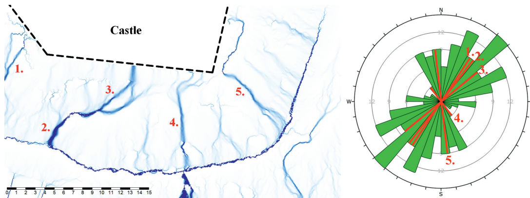
Fig. 2. New Figure: Fig. 12. Joint system obtained by RPAS (marked on catchment area DEM) and also measured on the field. Numbers refer to major joint systems marked on DEM map and on rose diagram
