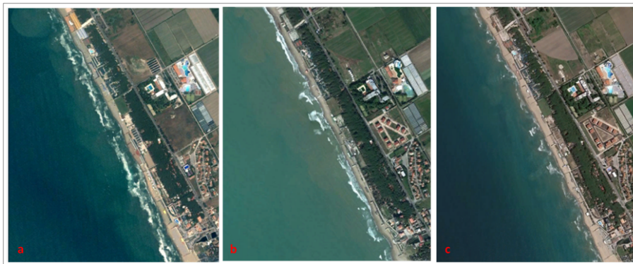
Figure 6. Evidence of rip-currents in Google Earth™ images a) 28/06/2007 (Image©2016 European Space Imaging); b) 02/05/2013 (Image©2016 Digital Globe); c) 29/05/2015 (Image Landsat/Copernicus).
