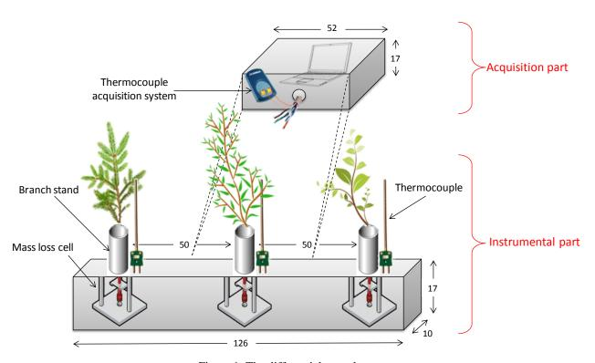
Figure 1: The differential mass-loss prototype
