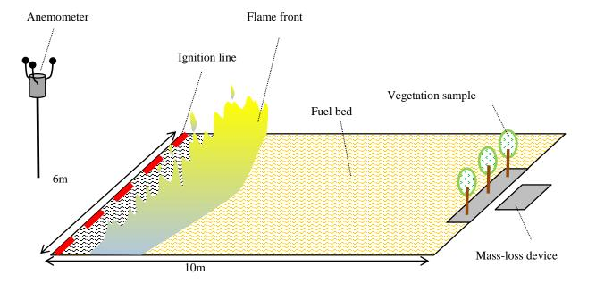
Figure 2: Experimental configuration
