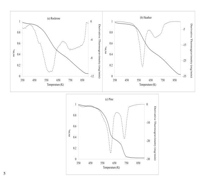
Figure 4: TGA (lines) and DTG (dotted) of oven dried of Rockrose (a), Heather (b), Pine (c) samples obtained with a linear heating rate of 30 K/min under air atmosphere.
