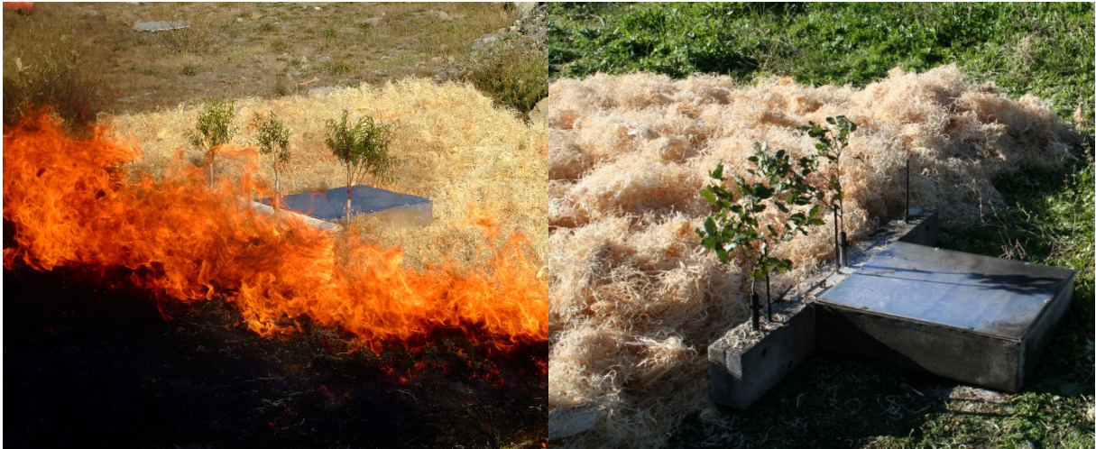
Figure 4: Differential mass loss prototype placed in the middle (left) and at the end (right) of the fuel bed.
