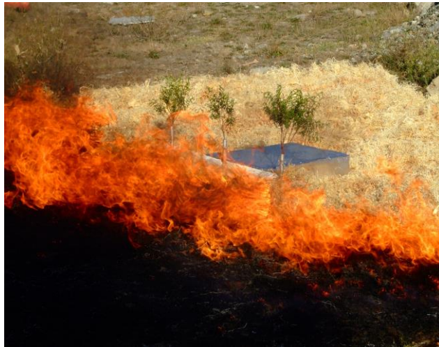
Figure 4: Differential mass loss prototype in field conditions
