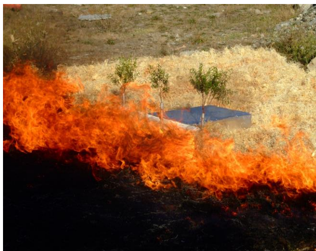
Figure 4: Differential mass loss prototype in field conditions
