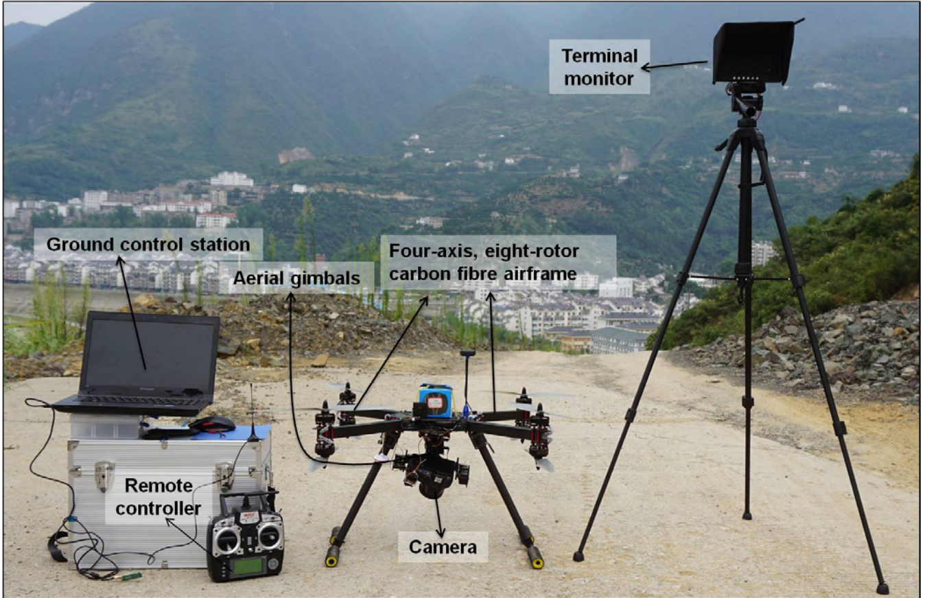
Fig.1. A photograph showing the customized UAV system used for emergency investigation of single geo-hazards in the Three Gorges Reservoir area, China.
