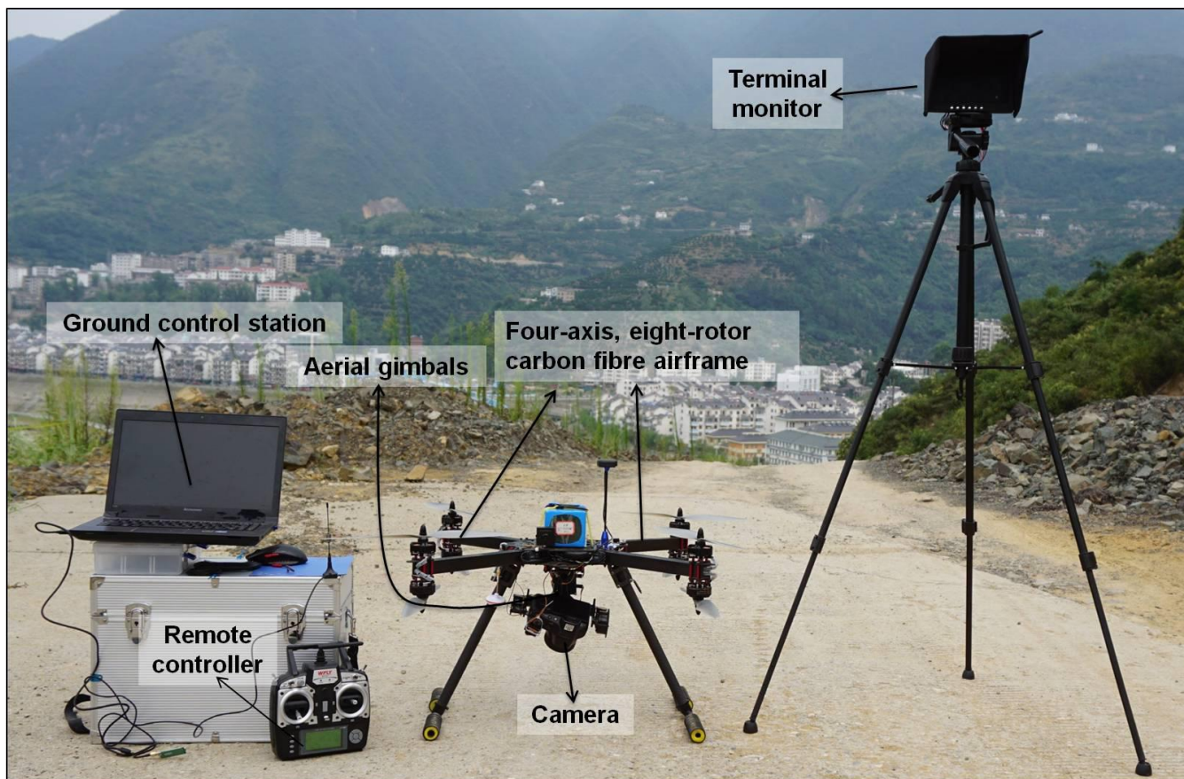
Fig.1. A photograph showing the customized UAV system used for emergency investigation of single geo-hazards in the Three Gorges Reservoir area, China.
