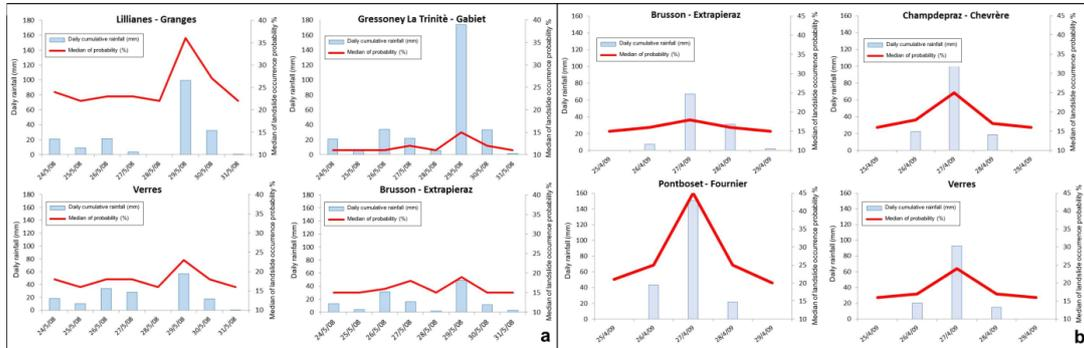
Figure 9. Correlation graphs between the daily cumulative rainfall and the median of landslide occurrence probability for both events.
