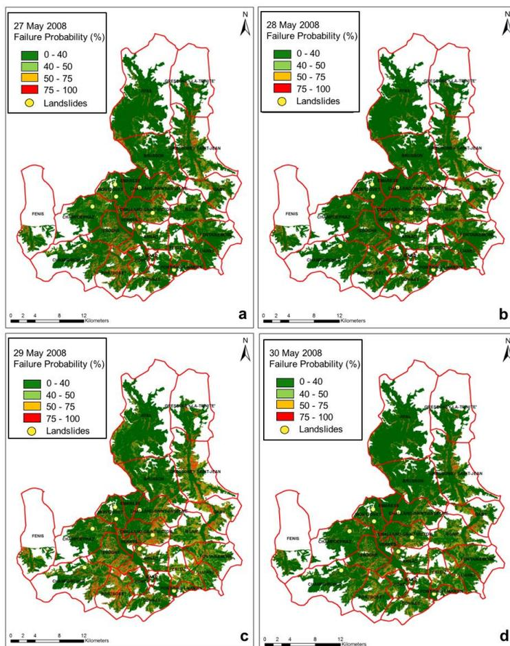
**Figure 7.** HIRESS landslide probability maps of simulate event of 24-31 May 2008 and reporting landslide during this event focused on the four critical days, a) 27 May 2008, b) 28 May 2008, c) 29 May 2008, and d) 30 May 2008.
