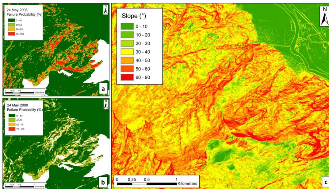
**Figure 6.** Example of numerical mask to remove the false positive of the first event simulated, between 24-31 May 2008, a) the HIRESSS result of the first day of simulation with false positive pixels, b) the probability map after the numerical mask implementation, c) the slope map shows that the pixels with high probability of landslide occurrence are located where the slope is higher than 60%.
