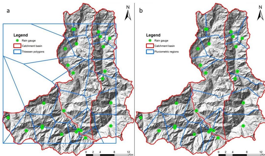
**Figure 5.** Comparison of Thiessen's polygons methodology a) simple b) modified according to the catchment basins boundaries.
