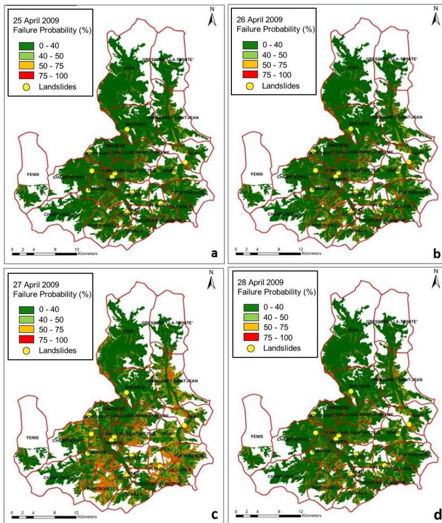
**Figure 8.** HIRESS landslide probability maps of simulate event between 25 - 28 April 2009 and reporting landslide during this event, a) 25 April 2009, b) 26 April 2009, c) 27 April 2009 and d) 28 April, 2009.
