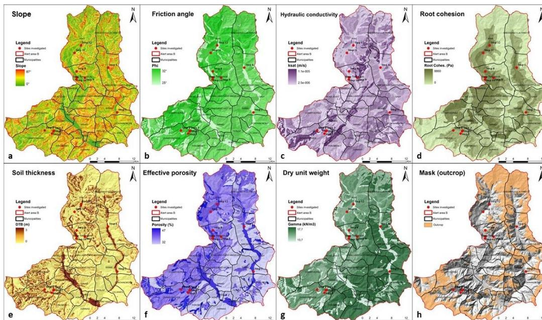
**Figure 4.** Static input parameters for HIRESSS model, a) slope gradient; b) root cohesion; c) friction angle; d) Hydraulic conductivity; e) soil thickness; f) effective porosity; g) dry unit weight; and h) exposure rock mask.
