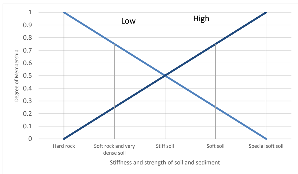
Figure 1. Fuzzification of stiffness and strength of soil and sediment
