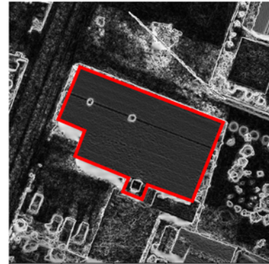
Figure 4: Gradient maps showing two buildings used to evaluate the horizontal accuracy of the DSMs. The cell sizes are the same as in the originals. Red lines indicate the edges of buildings or walls on the December 2015 map. Note that these lines are within high slope gradient areas on the maps for the other two dates. See Fig. 3a for the locations.
