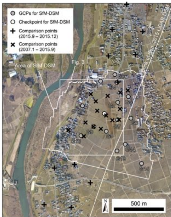
Figure 2: Distributions of GCPs and checkpoints for the SfM-derived DSM and comparison points for each DSM subtraction pair.
