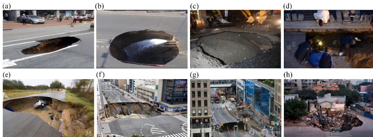
81 Figure 1. Ground subsidence nearby subway of urban railway: (a) Seokchon subway station, (b) Bakchon subway station, (c) 82 Samseongjungang subway station, (d) Janghanpyeong subway station in South Korea, (e) Texas in the US, (f) Fukuoka in 83 Japan, (g) Ottawa in Canada, and (h) Guangzhou in China.
