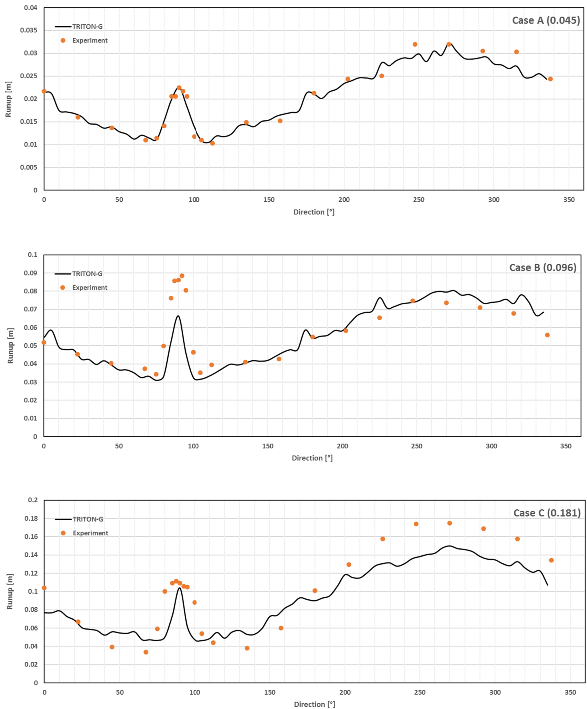
Fig. L Comparison between computed and measured run-up around the island for the three cases in BP6
