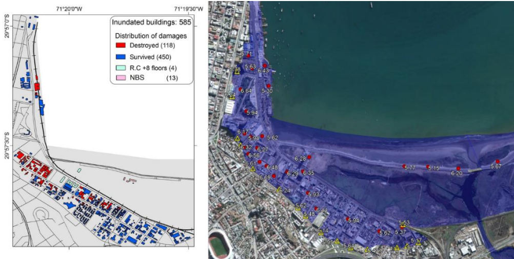
Figure 3. a) Surveyed damage to structures due to the 2015 tsunami. b) Coquimbo Inundated area (Aránguiz et al., 2016) and survey data.
