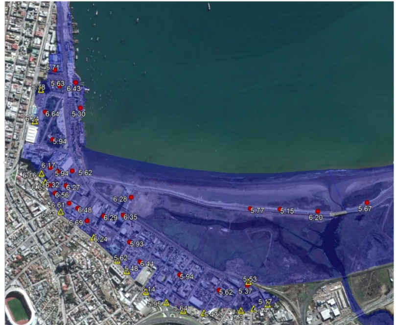
Figure 3. a) Surveyed damage to structures due to the 2015 tsunami; RC: reinforced concrete structures, L.S.: Light structures. b) Coquimbo inundated area (Aránguiz et al., 2016) and survey data. Red circles represent inundation measures and yellow triangles tsunami runup.
