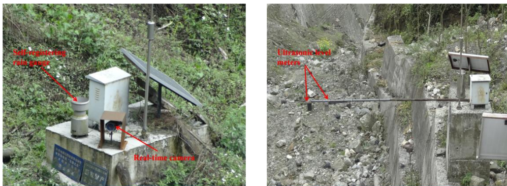
192 (a) Real-time camera and rain gauge (b) Ultrasonic level meters
