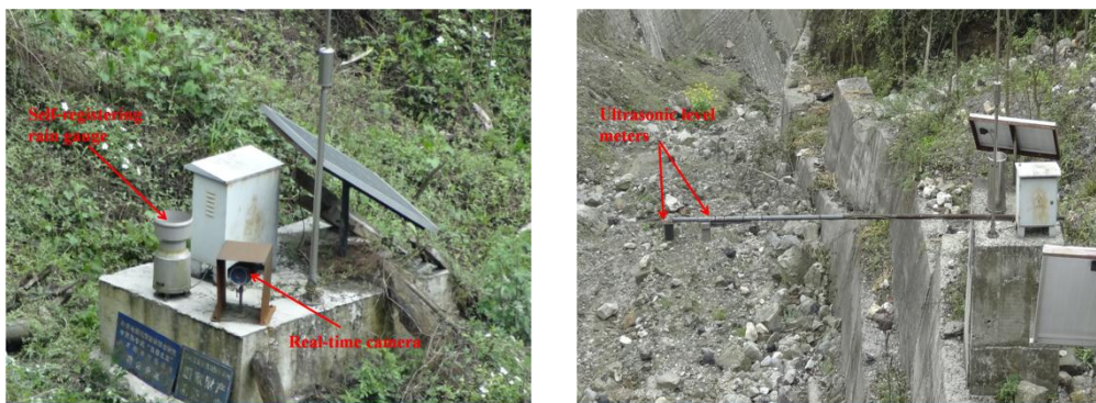
(a) Real-time camera and rain gauge (b) Ultrasonic level meters
