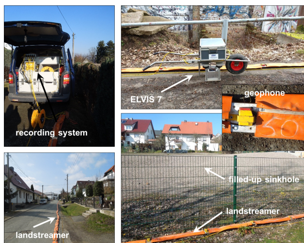
Figure 5. Photographs taken during the two field campaigns showing the micro-vibrator, the landstreamer and the recording system used for the S_H -wave reflection seismic surveys.
