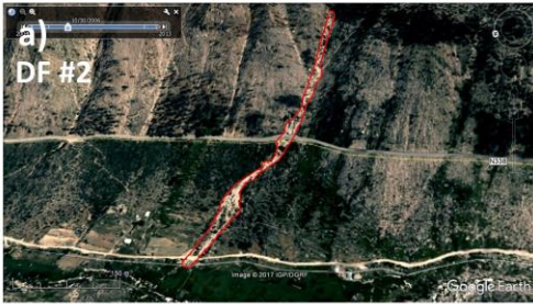
Figure 3. (a) Debris flows identification and delimitation; (b) Material deposited in the transport zone; (c) Deposits in the accumulation area.
