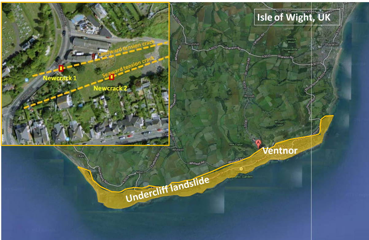
Figure 7: The layout of the Undercliff landslide and the position of crackmeters at location “A”.
