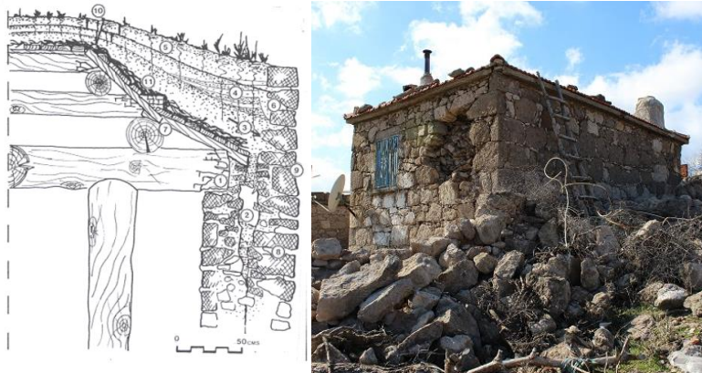
Figure 3: Typical wall construction detail (Hughes, 2000) and typical view of the a dwelling from the region
